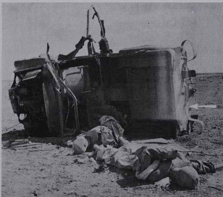
FIGURE 15. ROUND 3. CHAMP AT 2110 ft SHOWING DRIVER AND PASSENGER THROWN OUT OF VEHICLE
